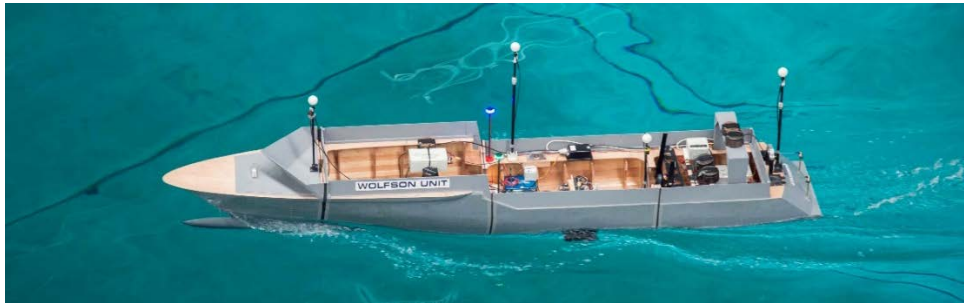
Figure 3 –Free running model fitted with motion capture markers during manoeuvring test in an ocean basins (photo courtesy of WUMTIA )
